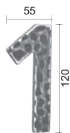
N. Spessore 4 mm. 0 Art. 16.022.12 1 Art. 16.022.13 2 Art. 16.022.14 3 Art. 16.022.15 4 Art. 16.022.16 5 Art. 16.022.17 6 Art. 16.022.18 7 Art. 16.022.19 8 Art. 16.022.20 9 Art. 16.022.21 Bloccaggio con 2 viti e tasselli da 10 Locking with no. 2 size 10 screws and expansion bolts
