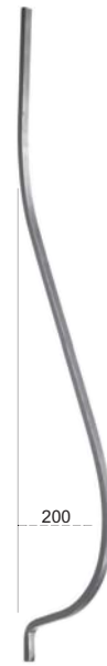
L.200 mm. □ 12 X 12 Art. 04.106.05 H. 950 mm. Art. 04.106.06 H.1200 mm. Art. 04.106.07 H.1500 mm. Art. 04.106.08 H.1800 mm.
